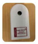
Water detectors are used to detect water leaks around the dialysis machine and around the water outlets for the machine. A water detector will also detect a blood leak from the dialyzer. Always sit a water detector directly beneath your dialyzer.
