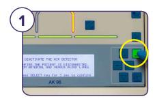
Press "SELECT" key for 3 seconds to deactivate the air detector.
