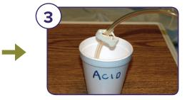
Place arterial blood line into a cup of acid concentrate and open clamp.
