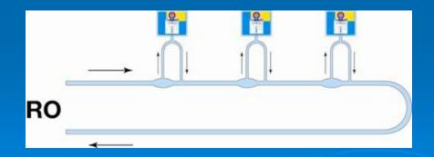
Tubing between ring main and HD machines must be integrated in routine disinfection.
