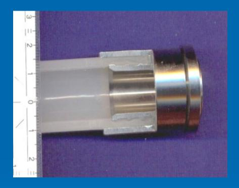
The design of a compression fitting includes dead spaces.
